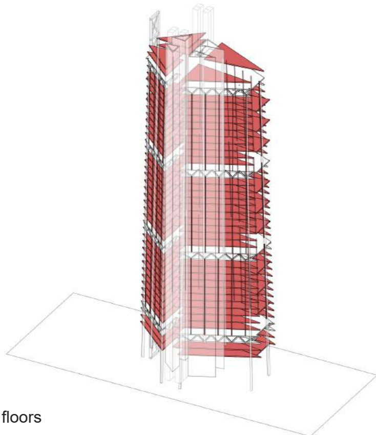
空心混凝土核心，垂直桁架梁和周边柱 Hollow concrete core, vertical truss beams and perimeter columns
